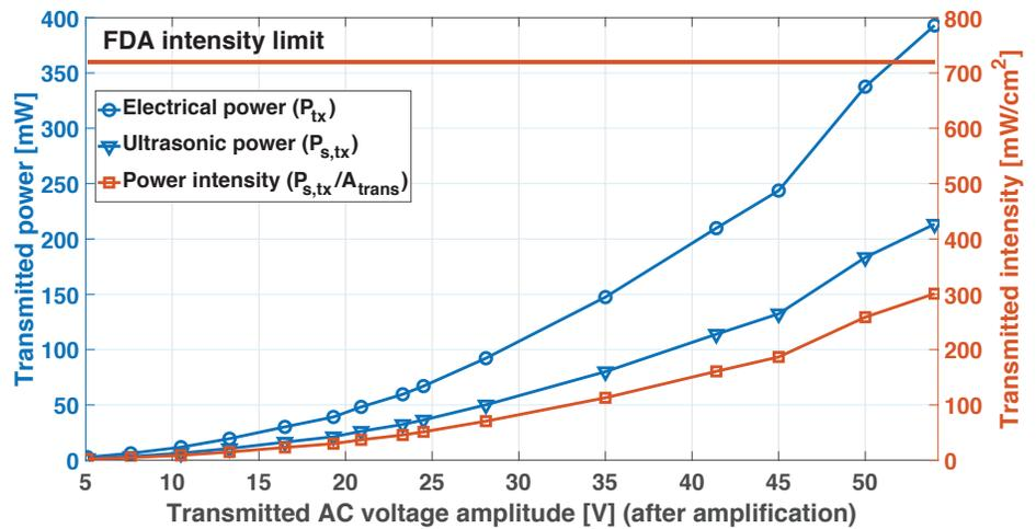
FIGURE 4. Transmitted power vs FDA limits.
