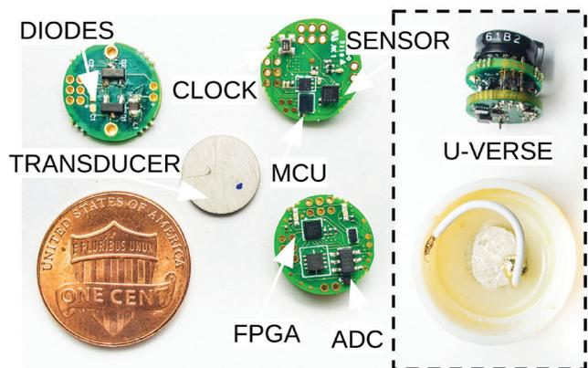
**FIGURE 2.** From top left, clockwise: energy harvesting unit (EHU), processing and communication unit (PCU) top and bottom side, penny, and ultrasonic transducer. The dashed box shows the full stack-up with a supercapacitor as power storage, as well as the transducer location.
