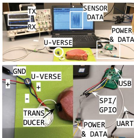
**FIGURE 5.** Closed-Loop U-Verse Application Demo.
