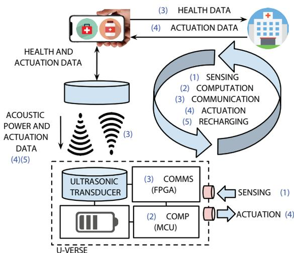
**FIGURE 1.** U-Verse enables end-to-end closed-loop long-lasting Internet of Implantable Medical Things applications.
