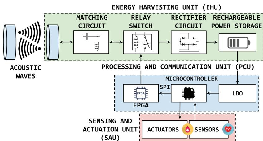
**FIGURE 3.** U-Verse is logically divided into an energy harvesting unit (EHU), a processing and communication unit (PCU), and a sensing and actuation unit (SAU).
